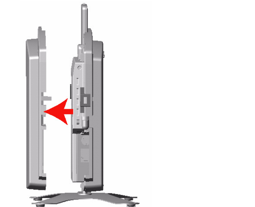
Figure 2-4 Remove the Front Cover
